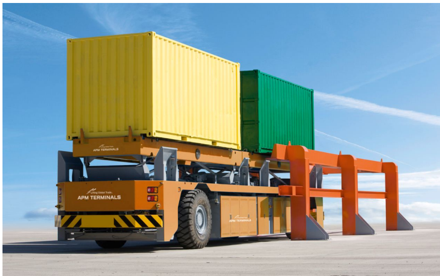
Figure 2.6: ALV with rack (Dredgingtoday.com).
