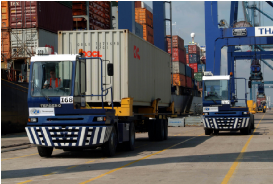
Figure 2.7: TT with chassis and container (Terbergenschop.nl).
